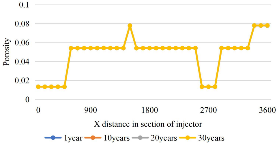
Figure 14—Sectional porosity distribution at different times in heterogeneous model overlaid each other.
